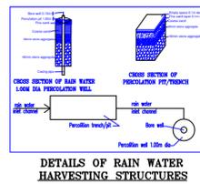
DETAILS OF RAIN WATER HARVESTING STRUCTURES
